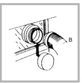
1. With a stacked dryer the hole in the window should ideally be made below the vent.
